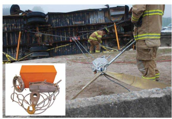
Individual Griphoist available in 1 ton to 4 ton capacity.
