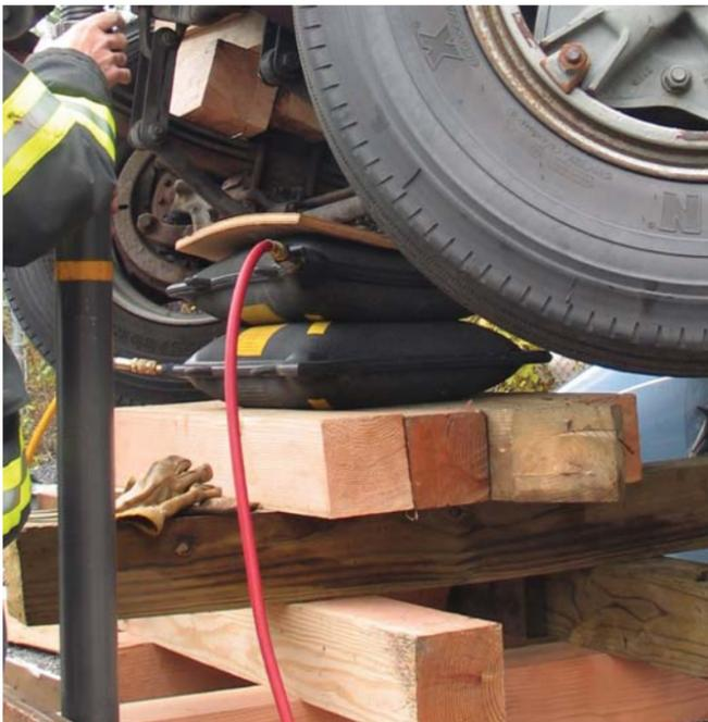
**1. Safety:** Maxiforce Air Lifting Bags are extremely tough, made of Neoprene, embedded with three (3) full layers of Aramid fiber reinforcement on each side, giving the bags tremendous strength at full inflation. Each Air Lifting Bag has been subjected to a stringent factory pressure test to assure maximum operator safety.
