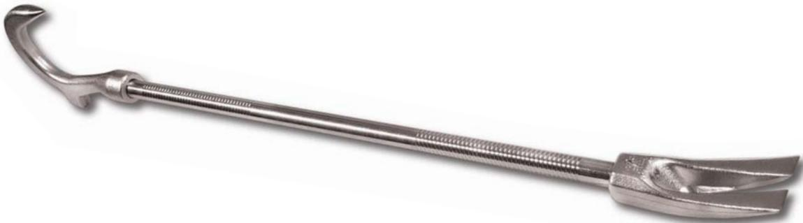
The Hook and Claw is a heavy duty prying tool designed for overhauling. Usually found on Ladder (Truck) Companies, the Claw Tool is very practical for prying floorboards, baseboards, window casements and door frames.
