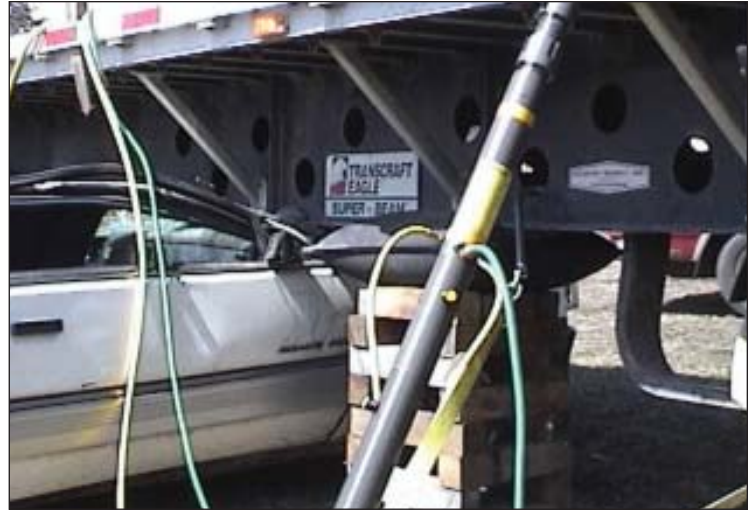
Maxiforce Strut and Air Lift Bags should be part of your road rescue equipment list.
